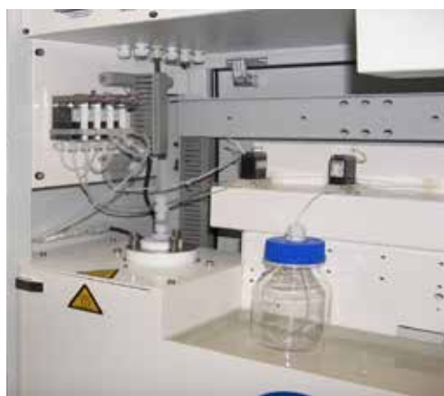
Figure 6: Quick-TOC-condensate with inject loop and inlet for wet standards or grab samples
