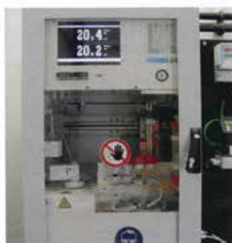
In contrast to laboratory methods, these analysers work automatically and detect quickly so that in the case of an alarm, any counter measures or trouble shootings are possible almost immediately.
